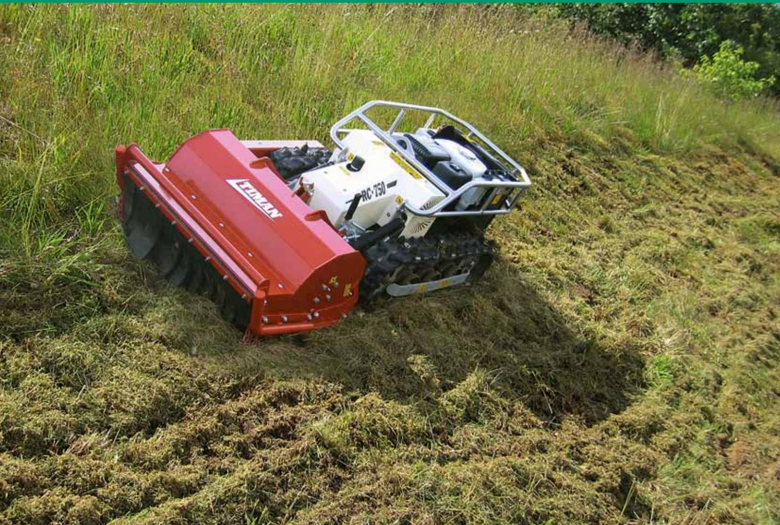
The out-front cut means that grass is cut before the tracks, and the full width cutting unit allows a close cut to walls and edges (especially on left hand side).
