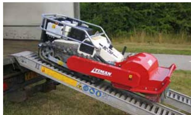
At only 330 kg gross weight, the RC-750 can easily be transported by trailer or lorry.
