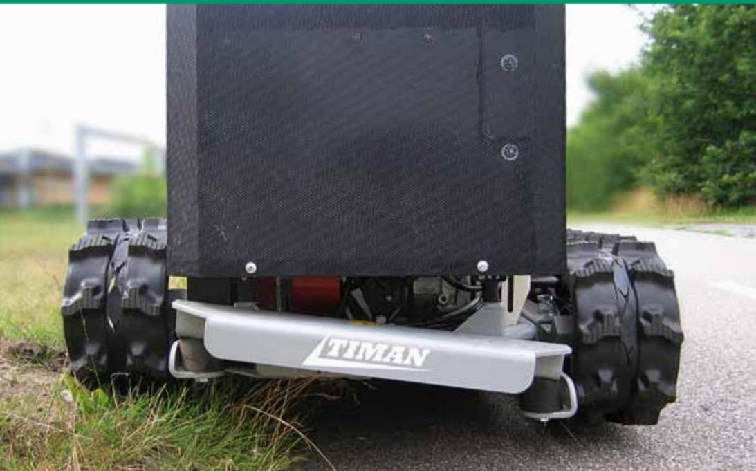
The two tracks are independently suspended, which means that the entire unit has always contact with the ground at four points, even on uneven terrains. This makes the device easy to control, as it moves steadily and has a good ground grip even on uneven surfaces.
